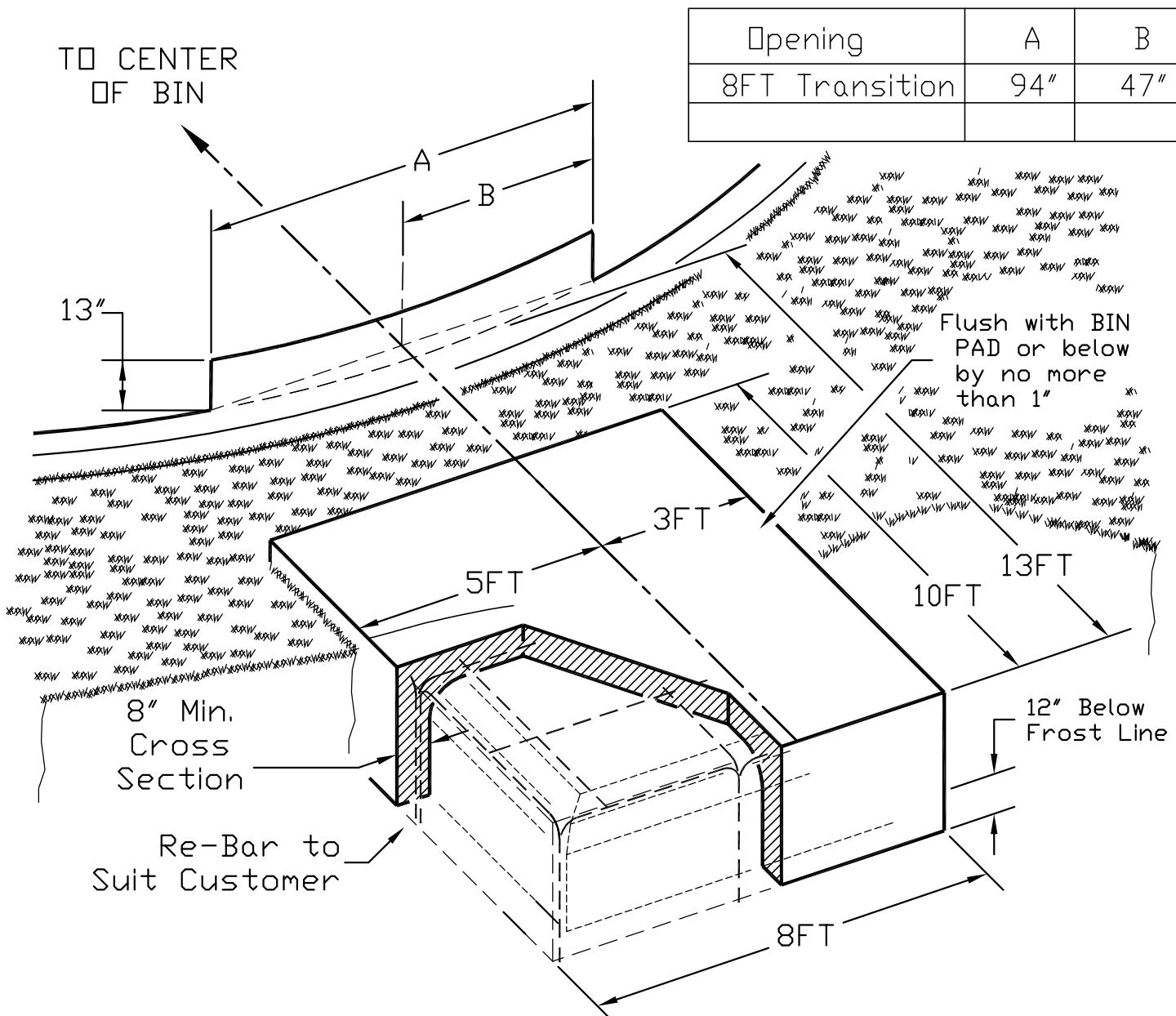
Note: The above drawing is what we suggest as a Foundation for your new Shivvers Dual Inlet Centrifugal Fan and Heater combination. We also suggest the foundation(s) of the Fan/Heater(s) extend below the Frost Line.
