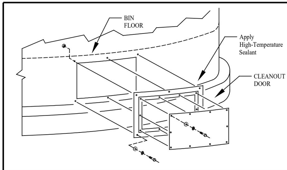
Cleanout Doors are most effective when used near the end of the drying season, when the bin is still nearly full. Do not even wait overnight as fines can draw moisture and set-up. When drying, shut off fan(s), open the Cleanout Door(s), turn fan(s) on, blowing dust and fines out of the bin. Turn fan(s) off, reinstall Cleanout Door(s), and finish drying.
