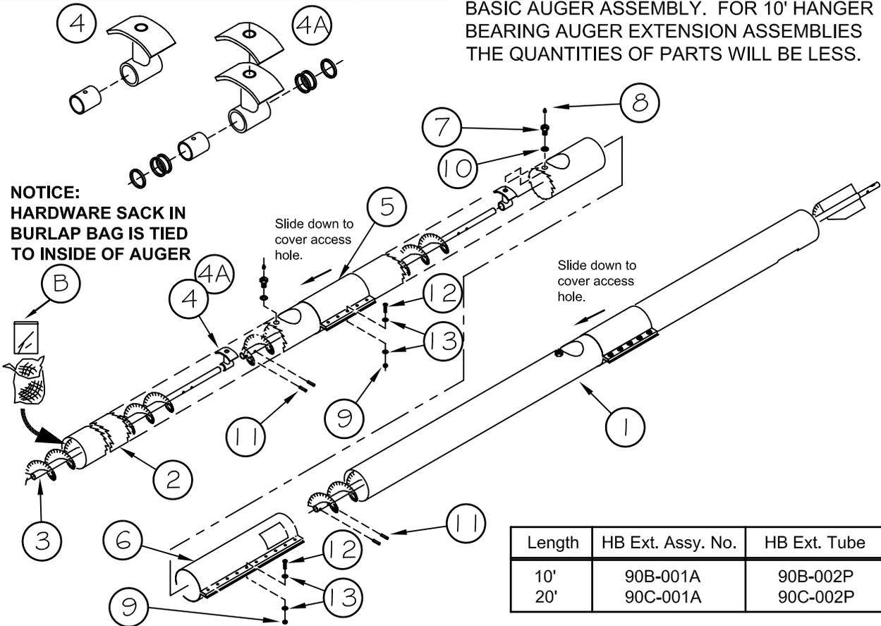
**NOTE:** All auger tubing must be butted tightly together and aligned before tightening the large connector sleeve. Proper alignment will help prevent premature excessive wear of the auger tubing.
