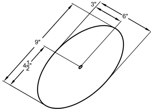
Elliptical Roof Hole for 6"
