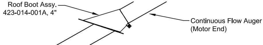
11. Install additional Roof Braces as required so that the auger is not unsupported for any span greater than 20 feet. (Refer to Step 5. Assemble Bipods in like manner.) A ground-based support or a truss assembly **MUST** be used where spans between any unsupported section are greater than 20 feet.
