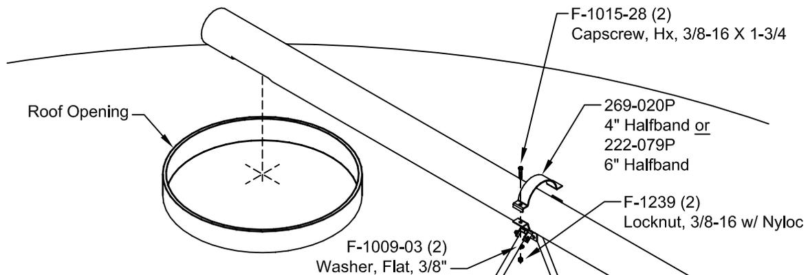
INSTALLING HOPPER: For Regular Hopper (Refer to P-11000 Super Hopper Installation Manual for installations using the Super Hopper.)
