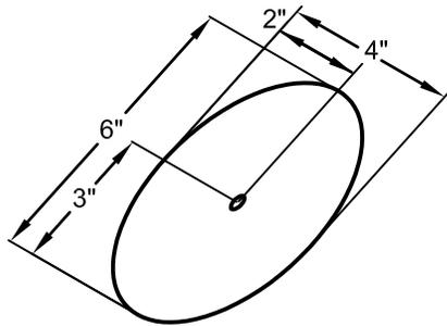
Elliptical Roof Hole for 4"
