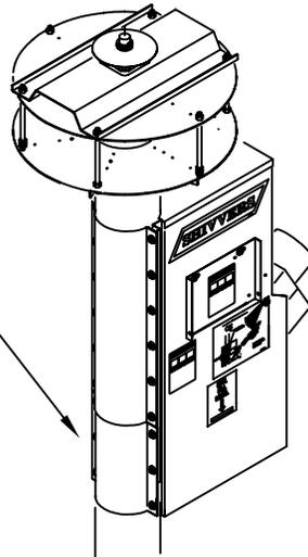
4. If it is necessary to align the Continuous Flow Boot to the storage bin, loosen the 4 Bolts on the Center Vertical Spreader Head Halfband directly above the Continuous Flow Boot. Rotate the Center Vertical Tube so that the Continuous Flow Boot points in the proper direction for the Continuous Flow Auger to exit the bin roof to the storage bin.
