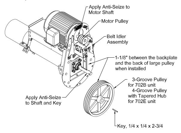
Apply Anti-Seize compound to the Motor Shaft. Install the Motor Pulley (ordered Separately), onto the Motor Shaft. Align with the large Pulley and tighten in place. Re-install the Outer Bearing Mount (removed earlier) onto the end of the Flipper Shaft and fasten it securely to the bracket on the Backplate Assembly. Tighten the
