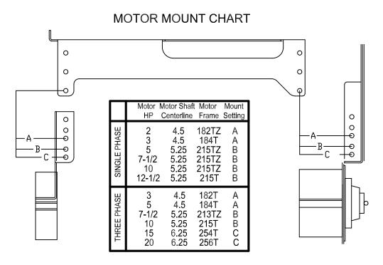
Install the Motor. (the center distance from the Motor Shaft to the Flipper Shaft should be about 15-1/4"\1/4") (Note: It is important that the Belt Idler Assembly is fully installed before installing the Motor, since the mounting bolt for it is trapped between the Backplate and the front of the motor.)
