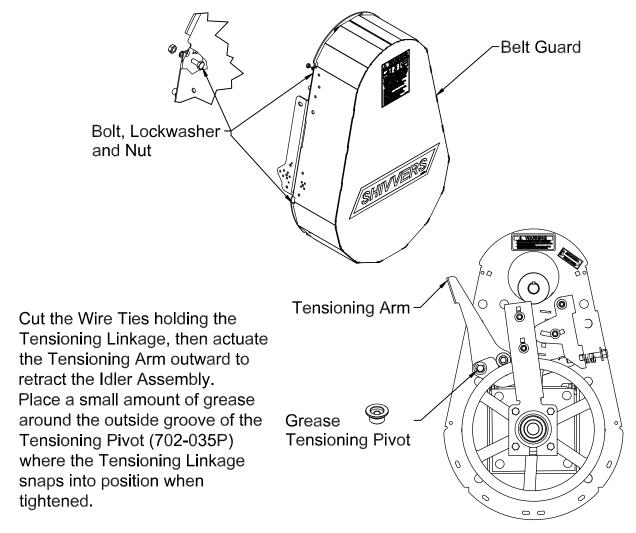
Install the Drive Belts D-3863 (BX62 Cogged Belts for 702B-001A) or D-3887 (BX64 Cogged Belts for 702E-001A). Note Clockwise Rotation.
