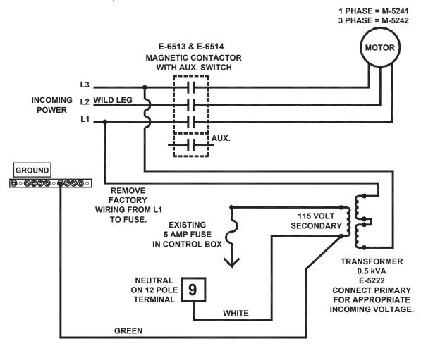
Remove factory wire from L1 to fuse. Connect wires from L1 and L3 to transformer primary. Put transformer jumpers in appropriate place for incoming voltage. Connect one pole of secondary to fuse. Connect other pole of secondary to both neutral (terminal #9) and ground lug. Remove fuse and apply power. Measure AC voltage across transformer secondary. It should be between 110 and 125 volts AC. Disconnect power and put fuse back in.
