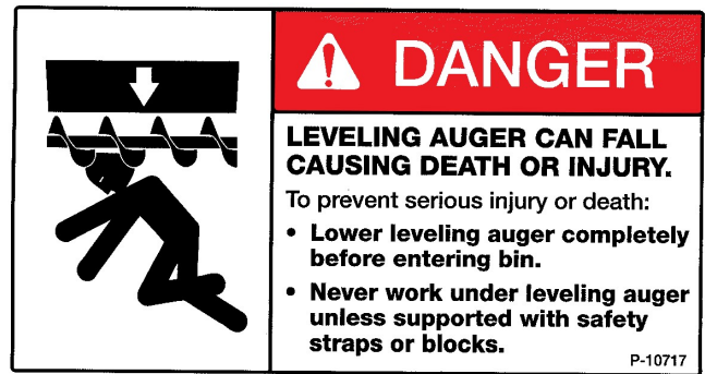
Figure: Leveling Auger Danger Decal
