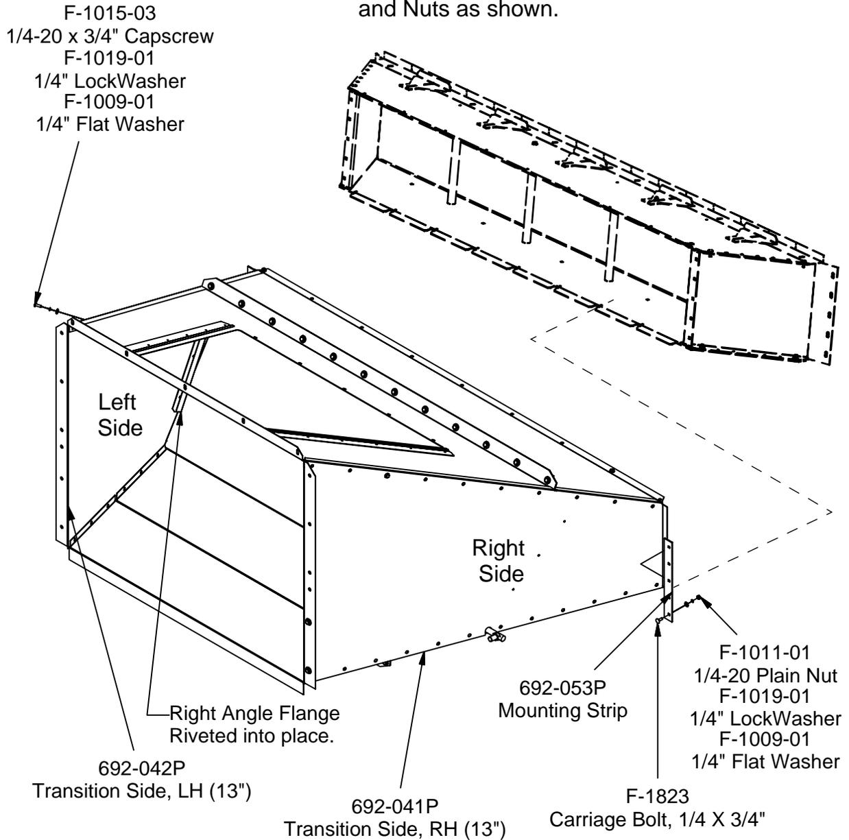
6. The Left and Right Side pieces (692-041P (LH) and 692-042P (RH)) fasten directly to the outside edges of the top and bottom with the U-nuts using 1/4" bolts, lockwashers and flat washers located in Hardware sack 692-056A. For both sides place the riveted right angle flange inward toward the damper door.
