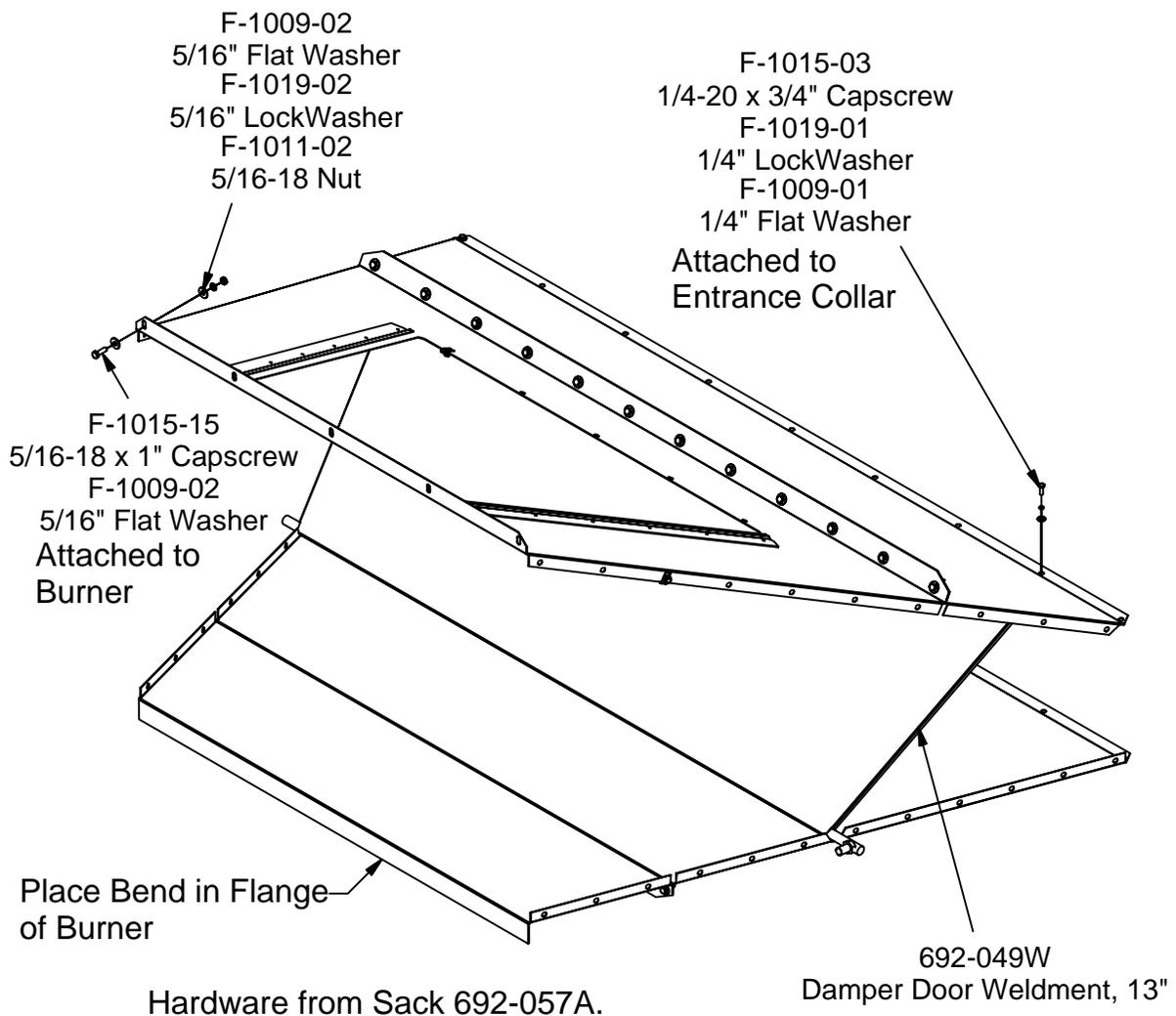
2 Connect bottom of transition to entrance collar with 1/4 x 3/4" bolts, washers and lockwashers fastened into U-Nuts. Place other end into groove in burner front.
