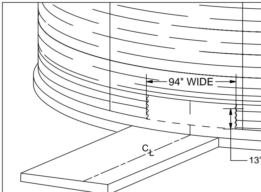
Cut a hole in the side of the bin offset over the fan/burner position approximately 13" x 94" wide.
