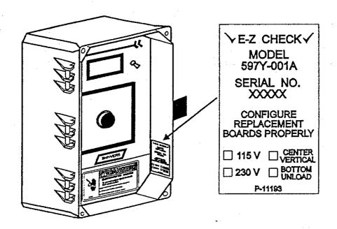
After the voltage and machine configuration have been set, be sure to mark the voltage and the machine type on the model/serial tag on the inside wall of the E-Z Check box. This will provide a record for future reference should the E-Z Check require any service.
