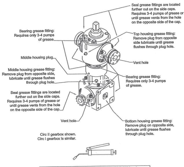
For standard (black, blue) Gearboxes use a Moly-Lithium base Extreme Pressure No.2 grease (NAPA Valvoline# 633).
