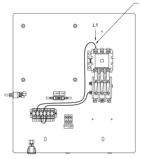
REMOVE THIS BLACK WIRE FROM L1 ON STARTER AND TERMINAL 2 ON TERMINAL STRIP.
