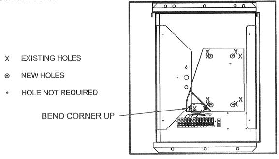
Step 8. Mount the pre-programmed ABB ACS150 V/F Drive (653-255A) using (4)
