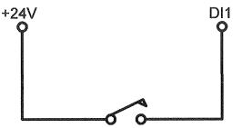
It may be necessary to use a wire nut and a short piece of wire if there is already a wire in the +24V terminal.
