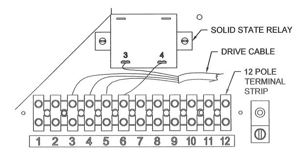
Step 5. Open the top door of the MVX9000 drive to locate the incoming power wires. Label and remove incoming power (top), and motor (bottom), wires attached to MVX9000 drive. Incoming power labels should be L1, L2 (if used), L3, and Ground. (There may be more than one wire under some terminals, just keep them together). Motor wires should be labeled T1, T2, T3 and possibly Ground.
