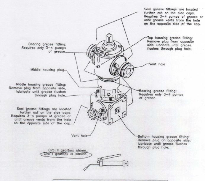
For standard (black, blue) Gearboxes use a Moly-Lithium base Extreme Pressure No.2 grease (NAPA Valvaline# 633).
