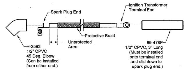
Press the elbow and 3" piece together. It is not necessary to glue them.
