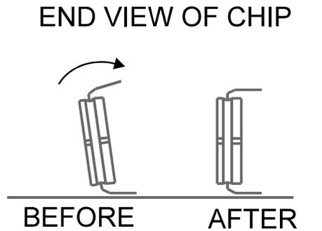
Place the chip in the socket making sure that the dot and or notch on the chip is pointing down and all the pins are in the socket. Using your thumbs, press straight down on the chip pushing it into the socket. Make sure all the pins are seated in properly. If a pin does get bent, the chip will need to be removed and the pin straightened.
