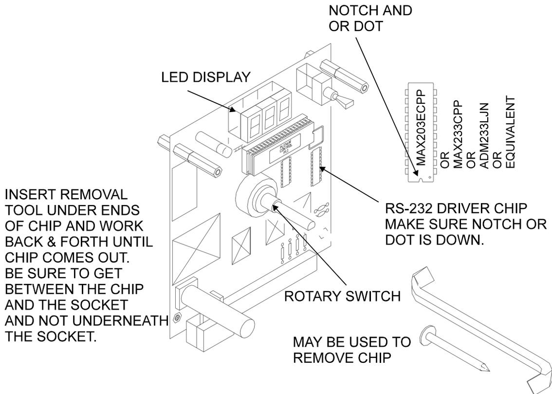
A tool will be needed to remove the chip from its socket. A small straight screwdriver will work. An offset flat screwdriver from NAPA, part # 374, or a 1½" roofing nail, may work, but may need some modifications made on a grinder. The tool needs to be thin enough to slide between the socket and the chip.
