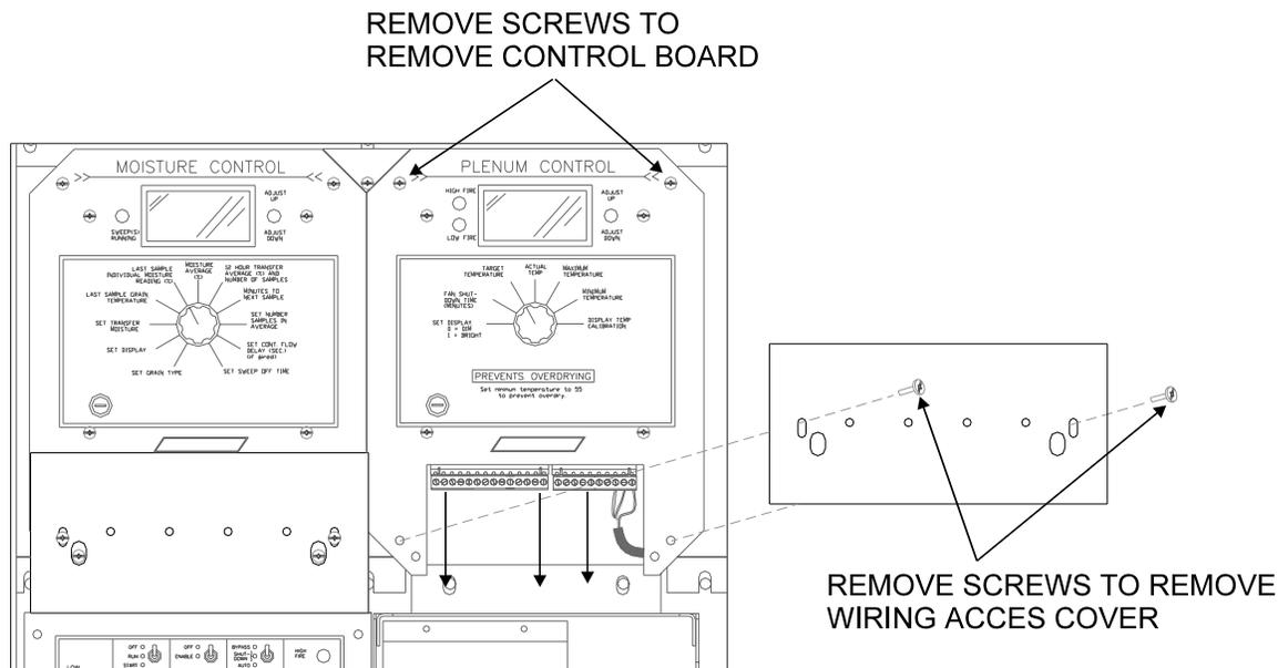
Once the control module has been removed from the command center or the E-Z Check, the faceplate will need to be taken off to gain access to the circuit board. Remove the knob by using a small straight screwdriver to loosen the set screw on the knob. The set screw is on the opposite side of the pointer. Loosen the set screw just enough for the knob to slide off. This will help to get the knob back to the right position later.
