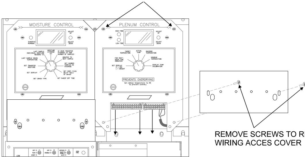
Once the control module has been removed from the command center, the cover plate will need to be removed to gain access to the circuit board. The knob will have to be removed first. Using a small straight screwdriver, loosen the set screw on the knob. The set screw is on the opposite side from the pointer. Loosen set screw just enough for the knob to slide off. This will help with getting the knob back on in the right position later.
