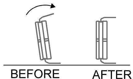
Place the chip in the socket making sure that the dot and or notch on the chip are on the right and all the pins are in the socket. Using your thumbs press straight down on the chip pushing it into the socket. Make sure all the pins are seated in properly. If a pin does get bent, the chip will need to be removed and the pin straightened.
