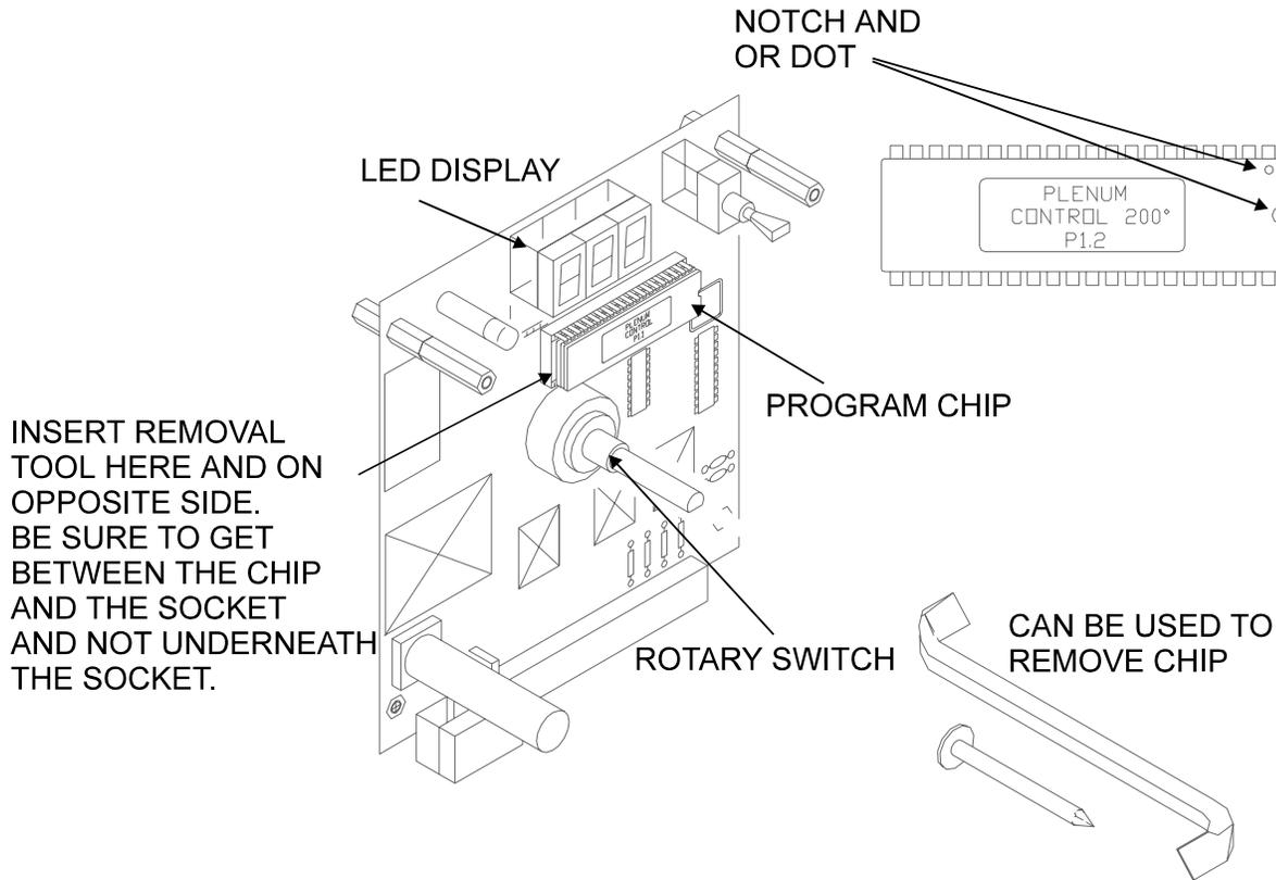
A tool will be needed to remove the chip from its socket. An offset flat screwdriver from NAPA part # 374 will work, or a 1½" roofing nail will also work. The tool needs to be thin enough to slide between the socket and the chip.
