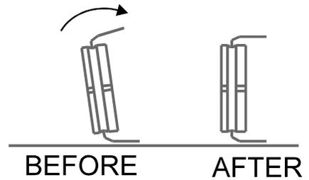
Place the chip in the socket making sure that the dot and or notch on the chip are on the right and all the pins are in the socket. Using your thumbs press straight down on the chip pushing it into the socket. Make sure all the pins are seated in properly. If a pin does get bent, the chip will need to be removed and the pin straightened.
