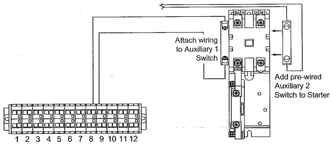
On some starter configurations it may be necessary to remove the auxiliary switch from the inclined fill auger starter. The auxiliary switch may also be moved to the other side of the inclined fill auger starter, if the starters are too close to each other.
