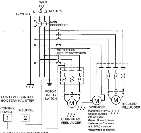
NOTE: Some 3 phase systems can't supply 115VAC when wired as shown. A Control Transformer (E-6353) will be required.
