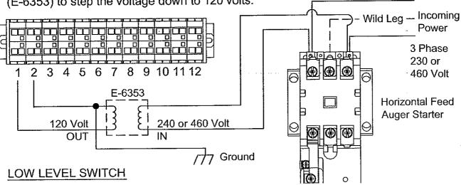
The Low Level switch should have closed contacts between terminals 8 and 9 without grain on the switch. The contacts should open when grain is present.
