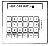
This allows entry of the starting plenum temperature. The Comp-U-Dry will adjust operating temperature as required. Range is 60 to 180° F but not larger than the maximum temperature. \*Default is last entry or maximum temperature.
