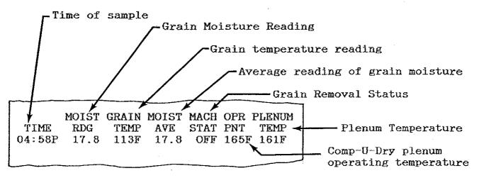
The average moisture content will be identical to the individual moisture sample on the first grain test. On subsequent samples, the average moisture content will reflect the average of the last four (4) or the operator selected number of sample readings to be averaged.
