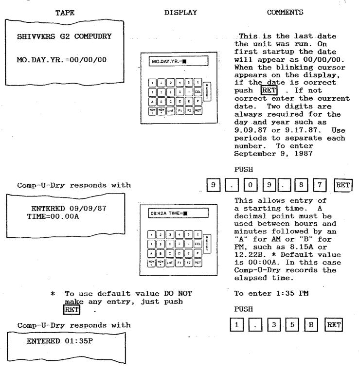
The only time the Comp-U-Dry asks for the time and date is on initial startup. While power is on, it will continuously update the clock. To change the time and date, shut power off, wait approximately one minute for the power supply to drain down and then turn the unit back on.
