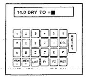
This allows you to select the grain transfer moisture. A decimal point must be used such as 14.0 or 14.6 and push RET to to complete entry. Range is from 8.0 to 29.9. Default value is last entry or 14.0.
