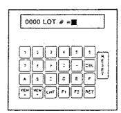
This allows you to identify the grain being dried for your records. Any combination of up to four letters or numbers may be entered. The Comp-U-Dry will automatically terminate after four entries. If less than four entries are made push RET after last entry. Default value is last entry or 0000.
