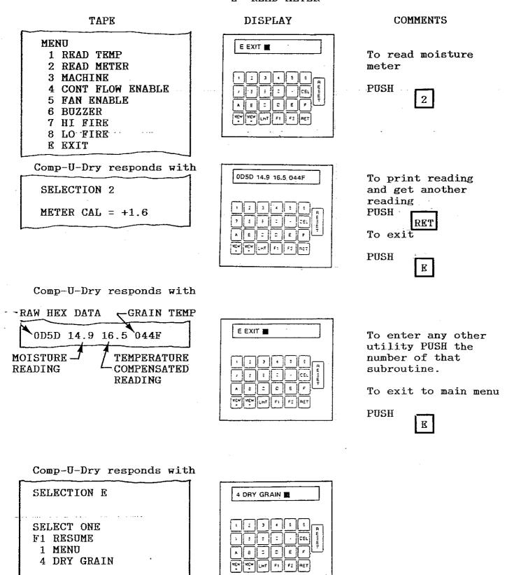
NOTE: Moisture readings will not be valid unless grain is moving through the auger.
