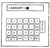
This allows confirming or changing the METER calibration. To confirm PUSH RET
