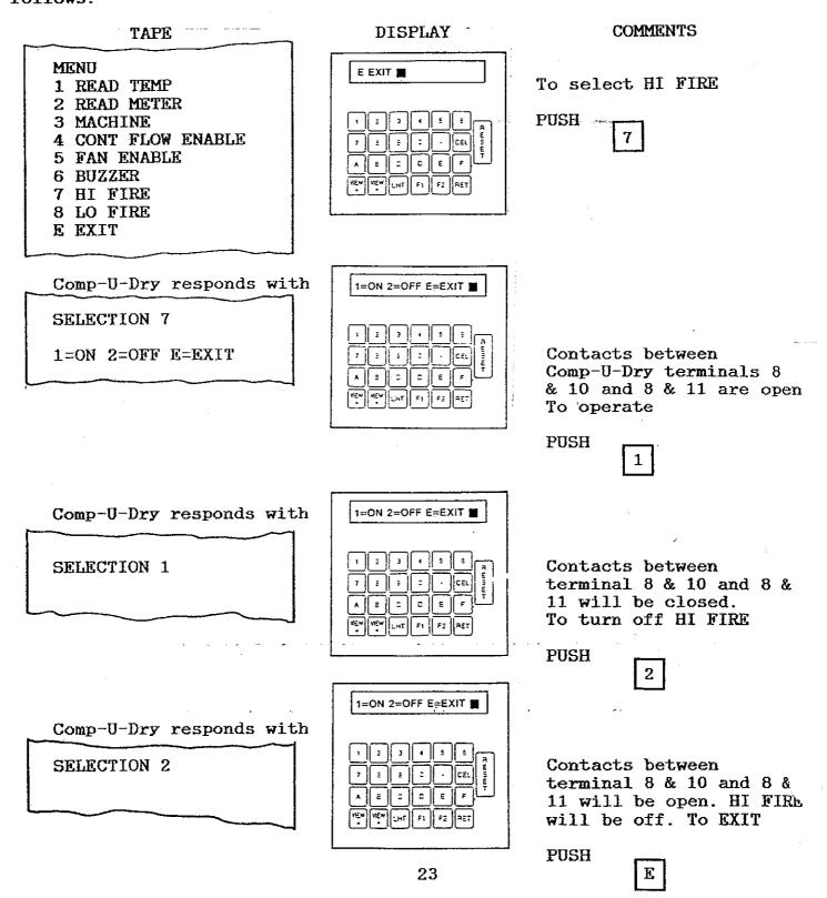
To operate the burner LO FIRE the Comp-U-Dry closes contacts between terminals 8 and 10 of the 16 point "F" terminal strip in the Comp-U-Dry.
