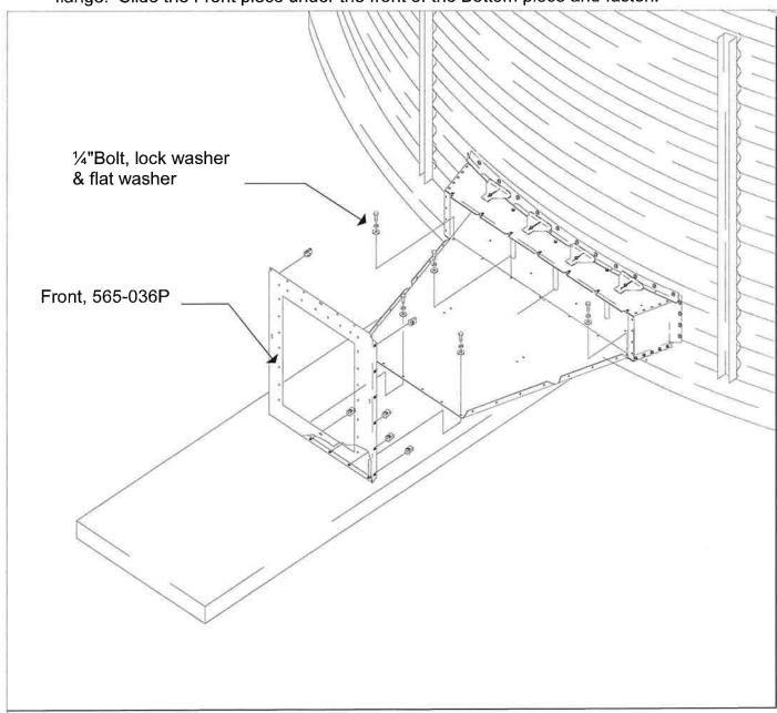
Place the Top Transition piece on the top of the Entrance Collar. Fasten with the ¼" bolts, lock-washers, and flat washers through the mating U-nuts on the Entrance Collar. Position the upper end of the top piece so that it lines up with the top of the Front piece. Using the U-nuts, "sandwich" the flange of the Top piece and Front piece inside the U-nut clip. Fasten using ¼"bolt and lock-washer only.
