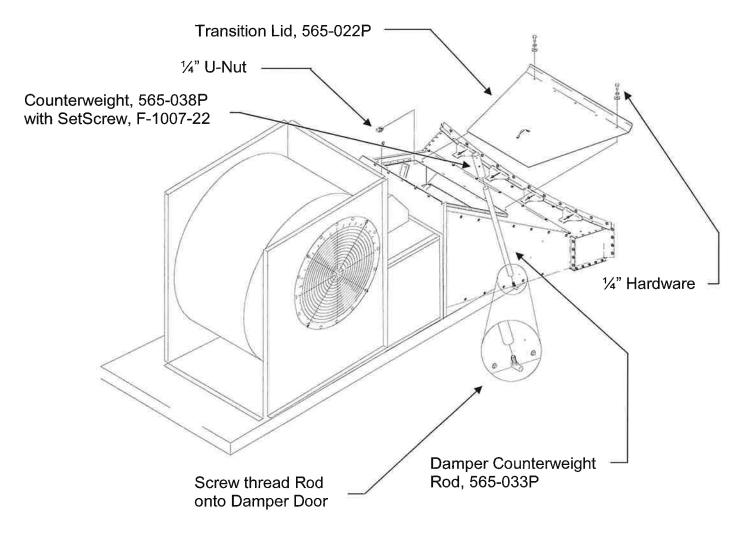
Slide the Transition Lid (565-022P) into the flanges on the Top piece. Use the  $\frac{1}{4}$ " hardware to secure the Lid through the U-Nuts.
