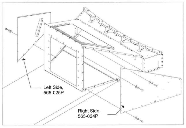
Locate the 565-037A Ent-Trans-Brnr Hardware Sack. This will contain all the hardware needed to fasten the Transition to the Entrance Collar and the Transition to the Burner.
