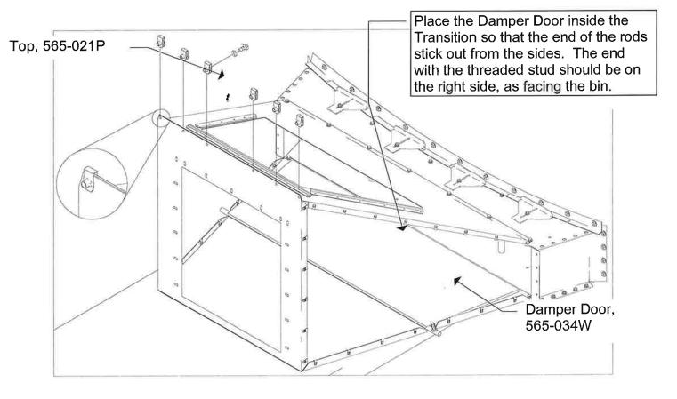
The Left and Right Side pieces (565-025P & 565-024P) fasten directly to the edges with the U-nuts using the ¼"bolts, lock-washers, and flat washers. For both Sides place the riveted right angle flange inward toward the Damper Door.
