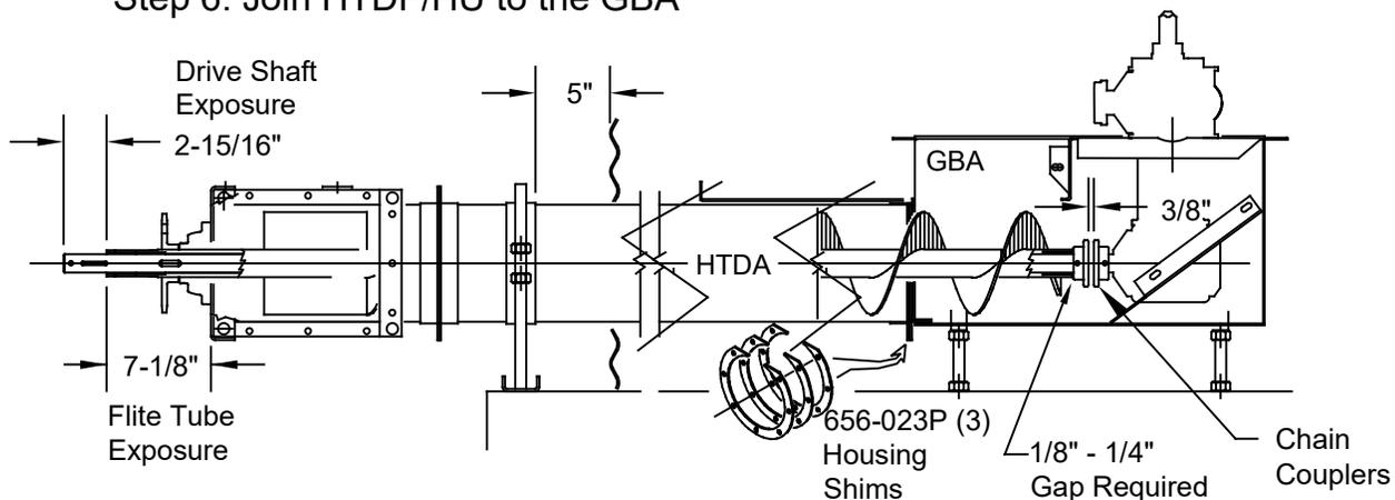
Positioning of the HTDF/HU housing is critical to prevent binding and misalignment. Pre-Assembly is necessary to determine the number of housing shims required.
