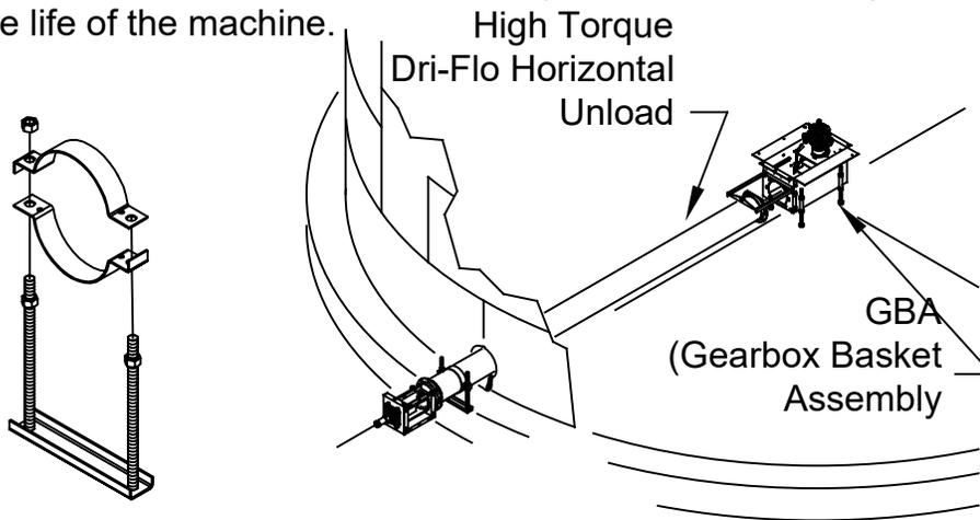
Assemble and Install a second mounting stand onto the HTDF/HU. This should be clamped to the tube at about halfway between the GBA and the bin wall. Make sure the location will not interfere with any intermediate wells. This stand is to support the HTDF/HU during installation, leveling, as well as for the life of the machine.
