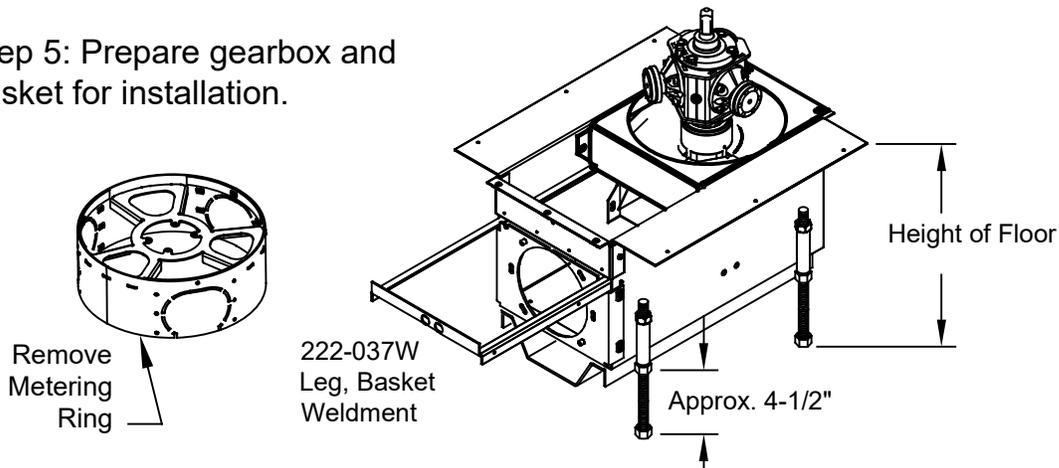
Remove Metering ring by loosening bolts from the top of gearbox. Replace lockwashers and bolts back into gearbox. Check the gearbox to insure it is lubricated. Remove the Shipping wire that holds the top gearbox to the bottom gearbox. Screw jam nuts, from 222-085A Basket Hardware Sack, on the 3/4"x 12" support legs at approximately 9". Screw the support legs, with the jam nuts, into the basket until the top of the basket will be about the same height as the drying bin floor.
