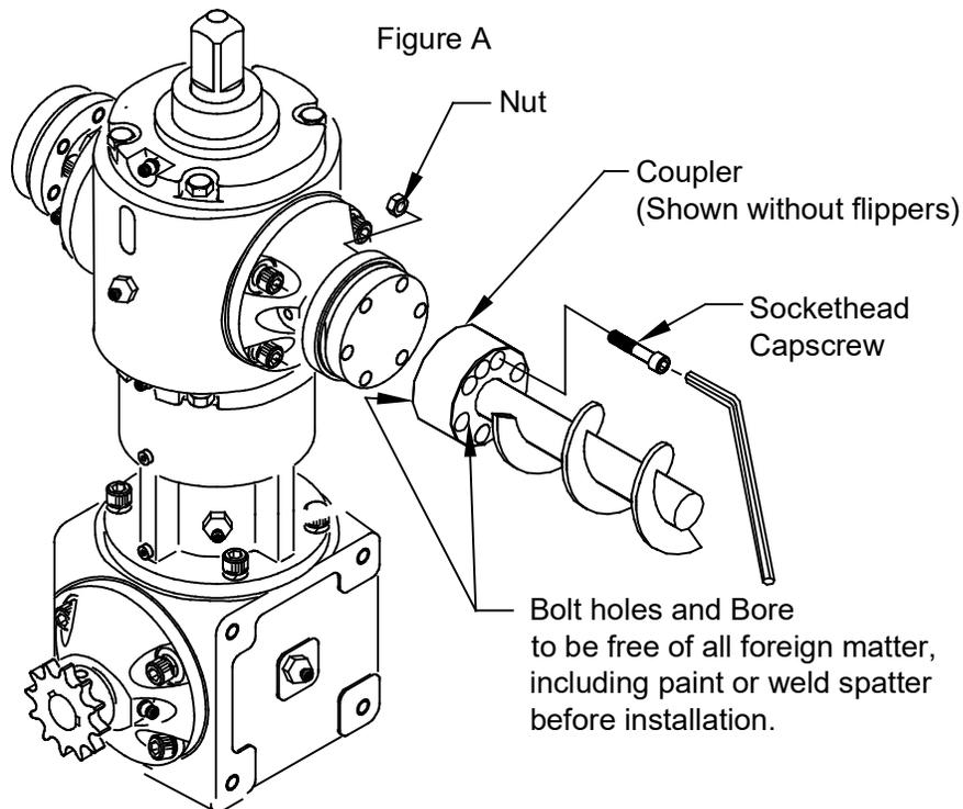
It is recommended that these bolts and nuts not be re-used. See your dealer or Shivvers for replacement of hardware sack #635-014A for 3/8 hardware or #712-010A for 7/16 hardware.
