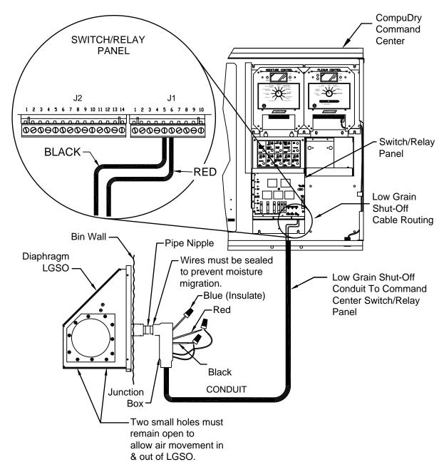
NOTE: Grain could be up to 24" above the Diaphragm LGSO before it actuates. Less grain will be required above it, if the sweep auger has passed under the switch. The switch will release when the grain level falls to about the middle of the diaphragm.
