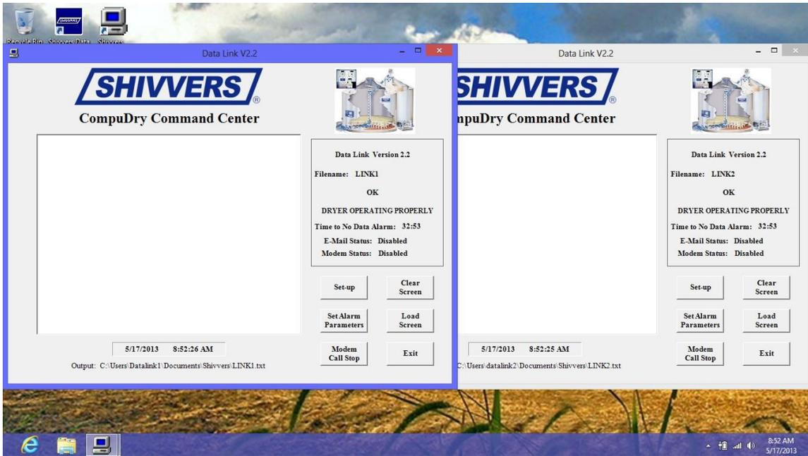
If the 232 adapters were switched, both of the Datalinks will throw errors. You can either switch the adapters or switch the com ports in both of the programs. This is why the adapters are marked and need to be kept in the same usb port.
