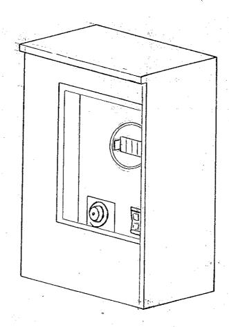
584A-001A 1 phase 5 HP. Max. 584B-001A 1 phase 7.5 HP. Max. 584C-001A 3 phase 7.5 HP. Max.
