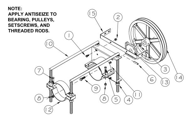
13. Attach the Downspout Assembly to the auger now, or after the auger is in place. The downspout assembly parts can be rotated to give different outlet angles.
