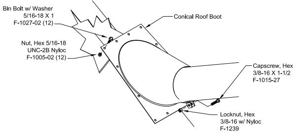
18b. (6" Only) Install the 2 Piece Roof Cone (423-373-001A) so that the long (slanted) piece is on top. Use the hardware from 273-092A, 2 Pc Roof Cone Hardware Sack found in parts box. Two types of fasteners are supplied for securing the roof cone to the bin roof. Use the supplied thum-seal to seal the edges and around the tube.
