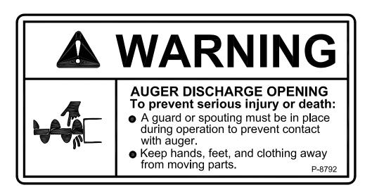
Located near discharge end of Continuous Flow and Auxiliary Transfer Augers (one on each side).
