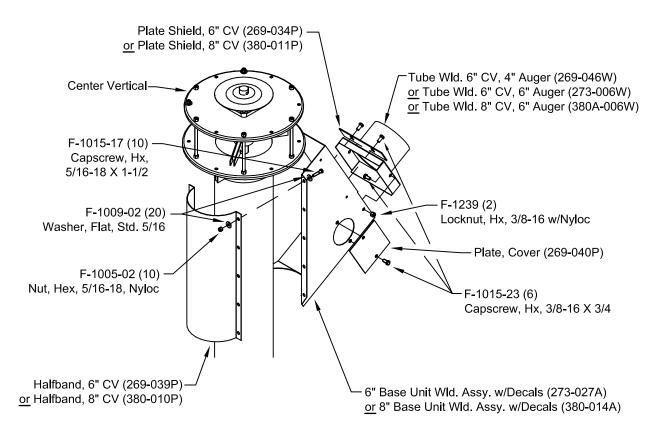
3A. Center the Continuous Flow Boot over the hole you have just cut in the Center Vertical. Mount into place and fasten securely with the halfband and hardware (269-014A, Boot Sack) provided with the Continuous Flow Parts box. Continue to Step 4.
