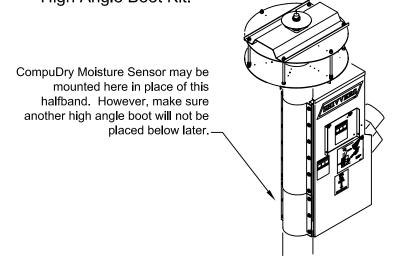
4. If it is necessary to align the Continuous Flow Boot to the storage bin, loosen the 4 Bolts on the Center Vertical Spreader Head Halfband directly above the Continuous Flow Boot. Rotate the Center Vertical Tube so that the Continuous Flow Boot points in the proper direction for the Continuous Flow Auger to exit the bin roof to the storage bin.
