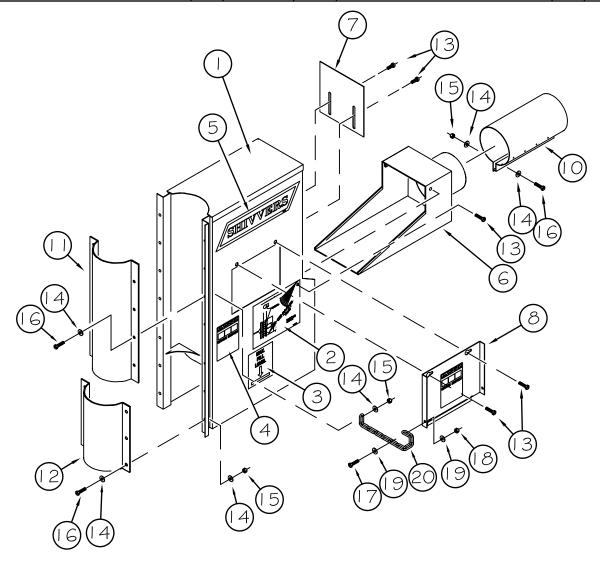
3B. Center the High Angle Boot over the hole you have just cut in the Center Vertical. Mount into place and fasten securely with the halfbands and hardware included in the HACV Boot Hardware Sack, 658-046A, found in the High Angle Boot Kit.
