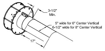
2A. Assemble the Continuous Flow Boot, as shown.
