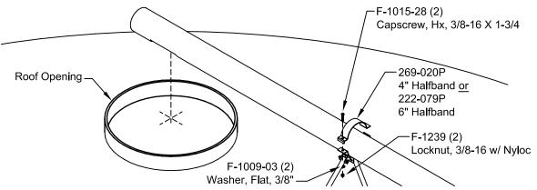
INSTALLING HOPPER: For Regular Hopper (Refer to P-11000 Super Hopper Installation Manual for installations using the Super Hopper.)
