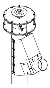
1B. For High Angle Boot only. Cut a hole in the Center Vertical tube for the Continuous Flow Auger High Angle Boot 6-1/2" wide by 14" long. The High Angle Boot can only be used with a 8" Center Vertical.
