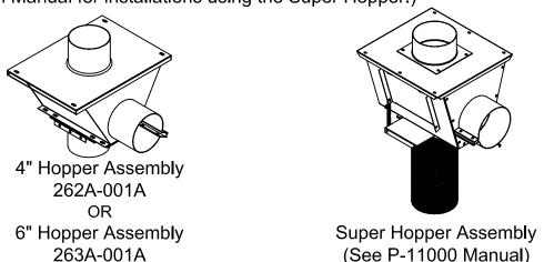
7C. Install the Hopper Assembly on the intake end of the tube, sliding the 1" shaft into the Plastic Bearing.
