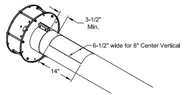
For High Angle Boot only 658P-001A, 8" CV, 6" Auger 658Q-001A, 8" CV, 8' Auger
