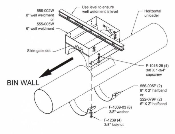
Insert the slide gate into the well weldment as shown. For a regular horizontal unloader, the center control rod hole of the well weldment is used. If a hanger bearing unloader is used, the offset hole of the well weldment is used (to allow grease zerk access). A six inch horizontal unloader always uses the center hole. Install cover plates over the unused control rod holes for an 8" well. A 6" well uses only one cover plate.
