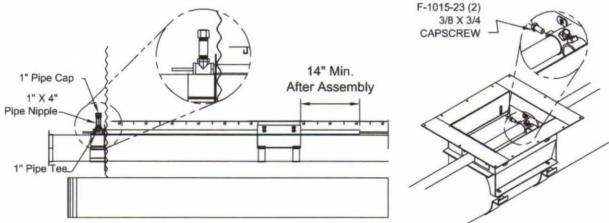
NOTE: Control Rods (two, 60" Long), 1" pipe tee, 1" coupler, 1" cap and 1" x 3"L pipe nipple available in kit #423-419-001A.
