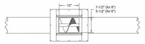
Position the well weldment with the slide gate slot pointing toward the bin wall (away from the gearbox) and attach it to the horizontal unloader as shown. Make sure the well weldment is level and tighten it securely in place.
