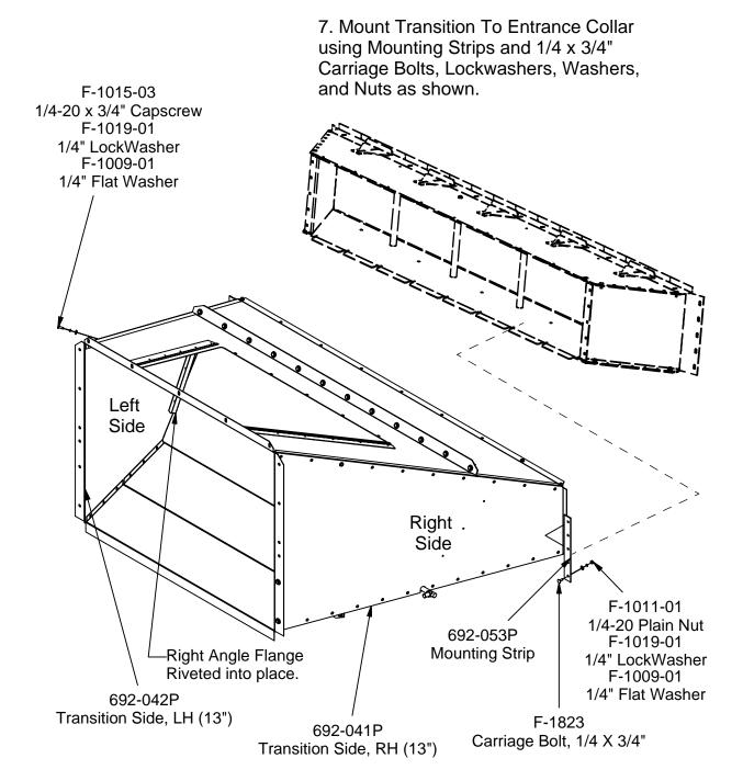
6. The Left and Right Side pieces (692-041P (LH) and 692-042P (RH) fasten directly to the outside edges of the top and bottom with the U-nuts using 1/4" bolts, lockwashers and flat washers located in Hardware sack 692-056A. For both sides place the riveted right angle flange inward toward the damper door.
