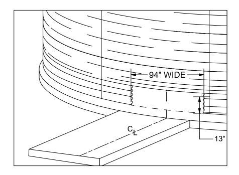
Cut a hole in the side of the bin offset over the fan/burner position approximately 13" x 94" wide. See Page 4 for Offset dimensions.
