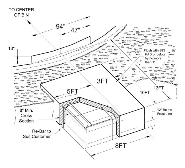
Note: The above drawing is what we suggest as a Foundation for your new Shivvers Dual Inlet Centrifugal Fan and Heater combination. We also suggest the foundation(s) of the Fan/Heater(s) be tied to the Bin Foundation, with all the foundations extending below the Frost Line.
