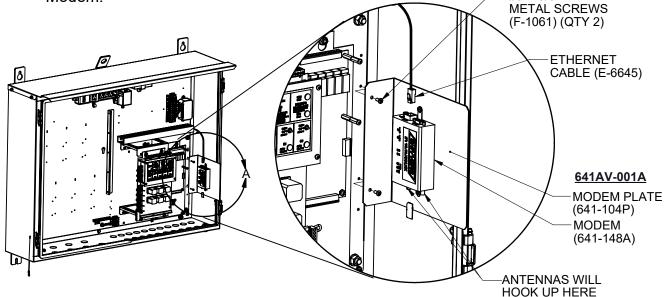
STEP 2. Slide the wire duct cover off. Route the power supply cord from the Modem through the wire duct and up to the power strip. Pull up any extra slack into the wire duct. Replace the wire duct cover.
