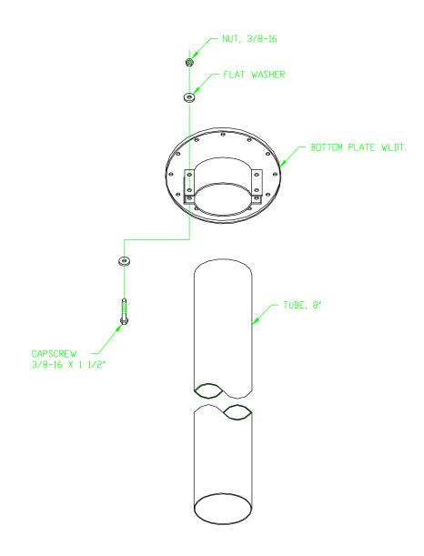
4. Slide the Level-Dry Center Tube Assembly onto the 8" tube from the other end. Put the 8" sleeve onto the 8" tube about flush with the tube end and secure with bolts, washers and nuts. Mount the 2 half-bands onto the 8" tube next to the sleeve.
