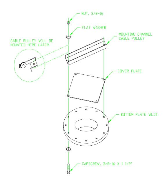
3. Slide the bottom plate all the way onto one end of the 8" tube. Tighten with 3/8" bolts, flat washers and locknuts.
