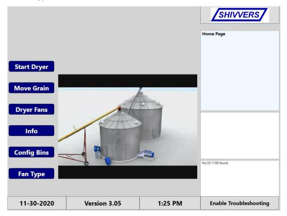
Press the Fan Type button, and a drop down box will open. Press on your fan type. Based on your fan type, static pressure alerts will be configured. Once you have chosen your fan type, press the Home button.
