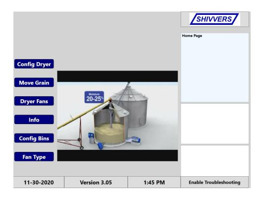
Note: After the dryer is initially configured, the Config Dryer button will change to Start Dryer. When Start Dryer is pressed, a pop up screen will appear asking if you want to skip settings or not. If you do not want to skip settings, the following pages are the same. The pop up screen does not appear when the button says Config Dryer.
