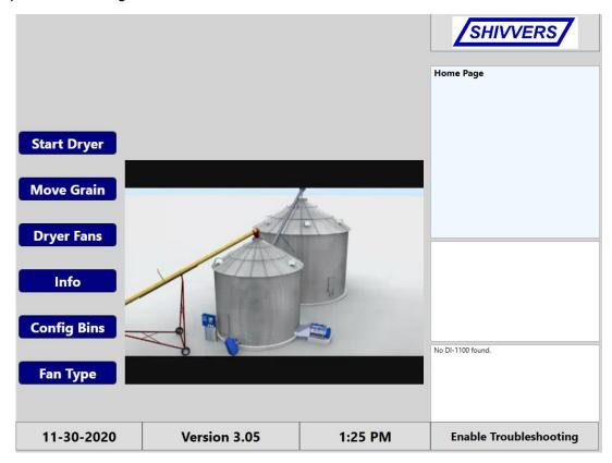
The next step is to set up the machine type, auger delays and storage bins. From the Home Page press the Config Bins button.
