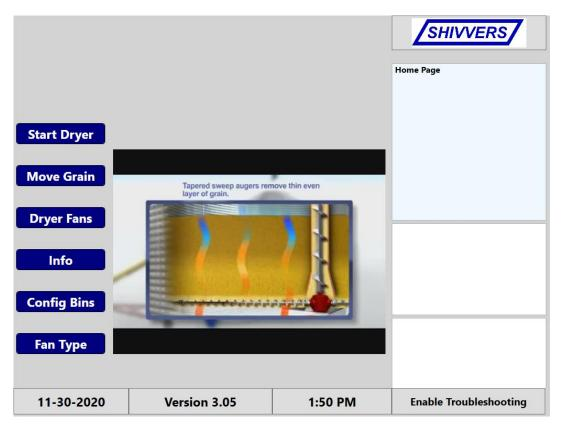
You will notice that the text of the top button has now changed from Config Dryer to Start Dryer. To start drying press the Start Dryer button. A pop-up message will appear asking if you would like to skip settings.
