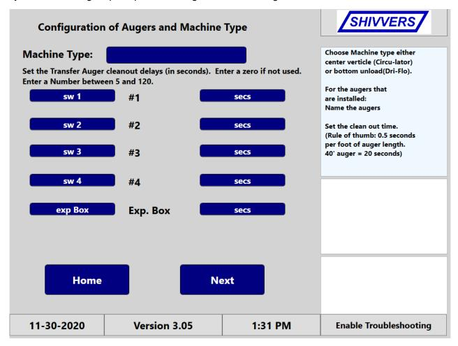
This is an example of how the augers and machine type could be set up for a center vertical.
